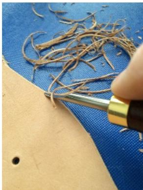
Now is a good time to bevel the edges of the leather on both sides and use the slicker on the bevelled edging.
