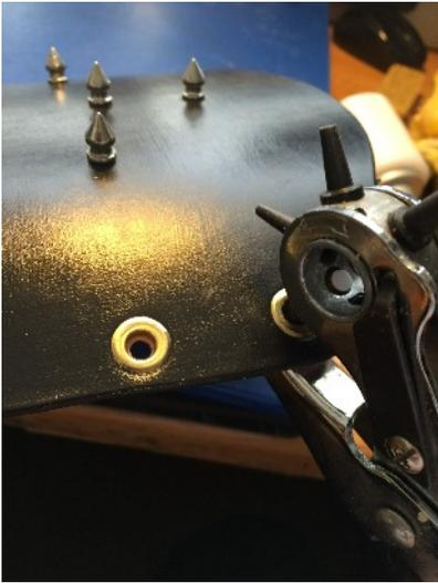
After riveting the material should be dry enough to finish the holes for lacing.
