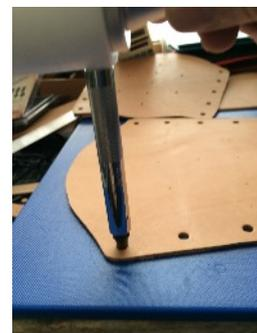
Setting out holes for spike rivets.
